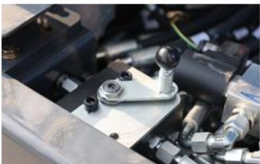
Forward/reverse switching valve
